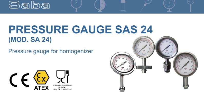
These instruments are designed for use on homogenizers for the food and pharmaceutical industry. Cushioned as standard, with internal shock absorber against pressure shocks, they are able to withstand high pressures repeatedly. The interstices-free construction and the degree of finish guarantee maximum hygiene.
